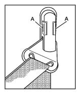
To move it up or down, squeeze the release buttons (A) together and move the height adjuster to the desired position. **Safety Belt Pretensioners**
